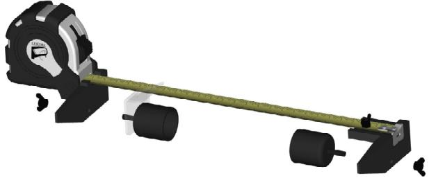
Fit the screw of the "thimble" into the hole in the tip and screw it in with the butterfly nut.
